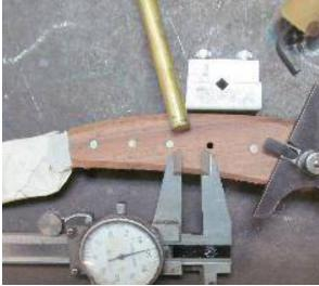
Use the drill press vise - clamp the handle parallel to the drill plane - align the bit over the hole (use an 1/8" as feeler gauge if unsure) and drill into the handle 0.25 to 0.375" deep - do NOT hit the tang. Flip it over and repeat on the other side.
