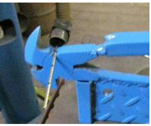
Shear the pins using a modified fence tool. Both ends are now distorted by the shear. Go to the grinder and grind a taper on one end of all pins.
