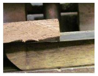
Repeat the process on the other scale. Place them around the tang and verify that there are no air gaps. If there are, you may have to deepen a recess or grind the tang a bit more.
