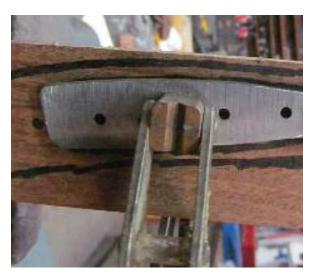
Since the scale is flat, a wood block can be used to create a horizontal plane over the drill press vise. A relatively narrow block (0.5"..0.75") is convenient and minimizes the number of times you have to reclamp. If you reclamp, be sure to use temporary pins and/or set another clamp before moving the first clamp. The tang cannot move relative to the scale. Drill the holes using the tang as a template.
