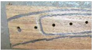
Measure the tang thickness at several spots along the tang. The thickest must be at the throat plane. If not - grind the tang until it is. The next step is to trace the tang onto the scale in such a way that you can easily see the outline.
