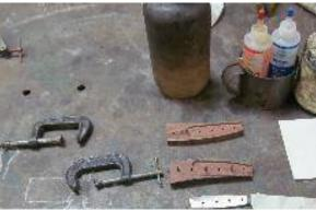
I like to have the center clamp on the opposite side of the handle from the other two clamps. Remove and wipe off the pins. Use a paper towel wetted with acetone and wipe off the throat area. Wait until the epoxy sets.
