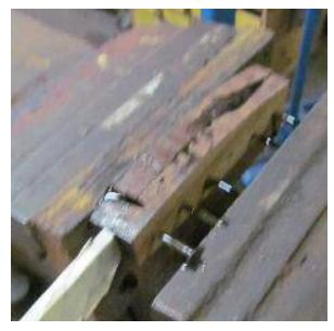
When done - make sure that all pins are proud on both sides. Let it set. When ready, grind off the protruding pins and epoxy splatter. Rough grind the edges of the handle to create 45 degree slopes but leave the pin area flat and hopefully parallel'
