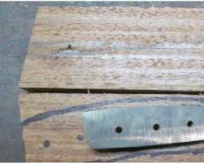
Position the tang on one scale and securely clamp it in place. If the tang has a significant dorsal to ventral taper, you can grind that somewhat flat back of the throat plane. When positioning the blade on the scale, make sure that there is no air gap between the back surface of the recess cut and the front surface of the block. It is better to have the wood surface slightly proud than leaving a gap.
