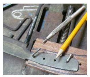
Go to the mill & etch-a-sketch out the recess by touching off the surface and then lifting the table 1/2 of the thickness at the throat plus 0.005". When milling the recess, go up to but not beyond the lines. It is better to leave a whisker inboard of the scribe line than going over the line. Remember - the closer the recess wall is to the tang, the better the probability of not seeing a cavity appear when grinding the handle.
